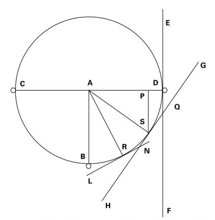
Fig. 2 Reduction of the inclined plane to the balance. Redraw from Galileo, De motu, Opere 1, 297.
