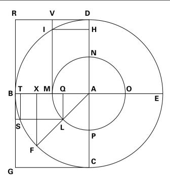
Fig. 1. Aristotle's mechanical principle. Redrawn from Alessandro Piccolomini, In mechanicas quaestiones Aristotelis paraphrasis (Venice, 1565), f. 15 r.
