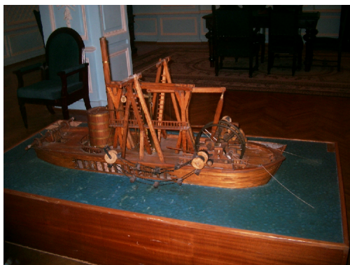
Fig. 3. A model of a steam-driven dredger (St-Petersburg University of Transport)
